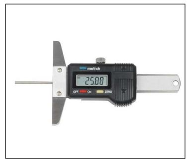
A digital depth gauge is a precision measuring instrument used for manual readings of displacement sensors including multipoint extensometers and crack gauges.
