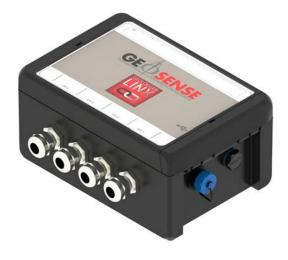
The GeoLogger Linx<sup>™</sup> is a range of low-cost battery-powered data loggers for stand-alone monitoring which can be used with all types of vibrating wire sensors such as piezometers, load cells, crack meters, joint meters, strain gauges, pressure cells, weir monitors and extensometers, together with their associated
