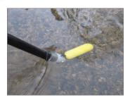
The Aqua-Data FloStick RC4 Water Velocity Meter is a standalone instrument comprising velocity probe, wading rod and display housing, all in a single integrated package. It uses the Faraday principle of electromagnetic induction and advanced analogue and digital electronics to offer an accurate, robust and low-cost method of measuring water velocity, and logging data for later analysis.
