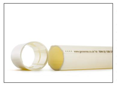
Geosense® XC (External Coupler) Inclinometer Casing is precision extruded from ABS, with four precise keyways formed at 90 degrees which allow accurate installation of portable and inplace inclinometers.
