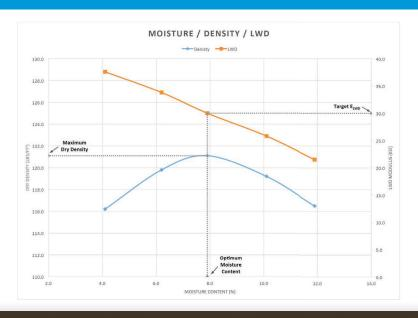
This plot shows how the optimum soil density/moisture content plot is used to establish the target soil modulus value,  $E_{LWD}$ , using the Olson LWD-Lab unit.
