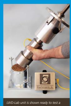
sample in a Proctor mold.
