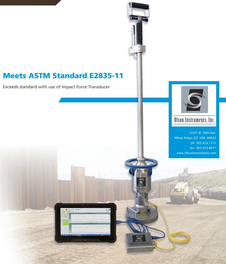
Measure Field Soil Modulus to Ensure Soil Compaction
