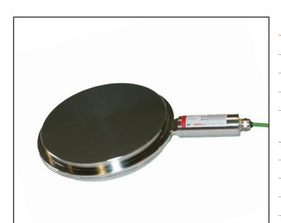
This consists of a sensitive pressure pad formed by joining two stiff steel discs at their periphery. The void inside the cell is filled with de-aired fluid. When load is applied to the cell the pressure of the inside liquid changes. The changes in pressure correspond directly to the load applied.
