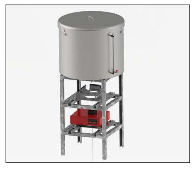
Geosense® HPS-3500 (Hanging) and IPS-3000 (Inverted) Pendulums are used to measure the tilt or rotation by measuring the relative internal horizontal displacement of points along a true vertical line. Each has a tensioned, stainless steel wire and the effects of the earth gravitational forces to guarantee a perfectly vertical line between a fixed point and a tensioning mechanism. Typical applications include concrete dams, bridges and high rise buildings.
