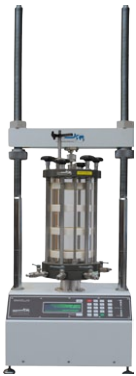
Traditional passive triaxial cell in 50kN load frame (100TC2)
