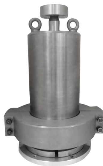
100MPa Triaxial Cell with 50mm max sample diameter (HP100MPA)
