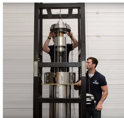
64MPa Active Triaxial Cell with Lifting Frame (HP64AC)
