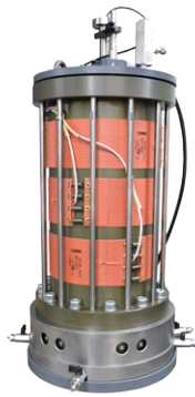
Traditional passive triaxial cell with heating elements (100TC4)
