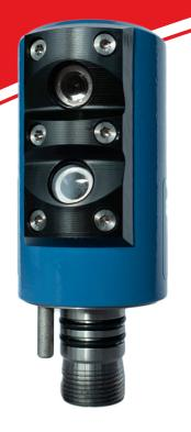
Turbidity Sensor 4296 is a compact fully integrated sensor for measuring optical backscatter in water. It is designed to be used with SeaGuard or SmartGuard data logger using AiCaP CANbus or as stand-alone sensor using RS-232
